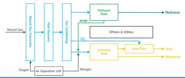
AdWinCombined™: up to 30% less CAPEX and approx. 10% less Feedstock consumption
